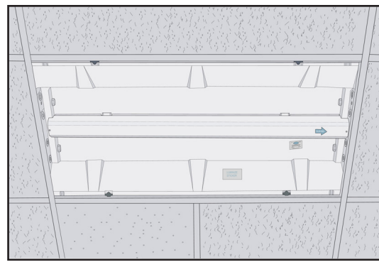
9. Install Notice sticker to inside of the fixture that can be easily seen when the cover is taken off.
